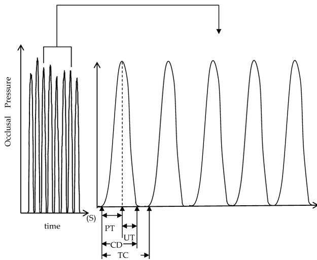
Figure 1. Occlusal pressure pattern while tapping
