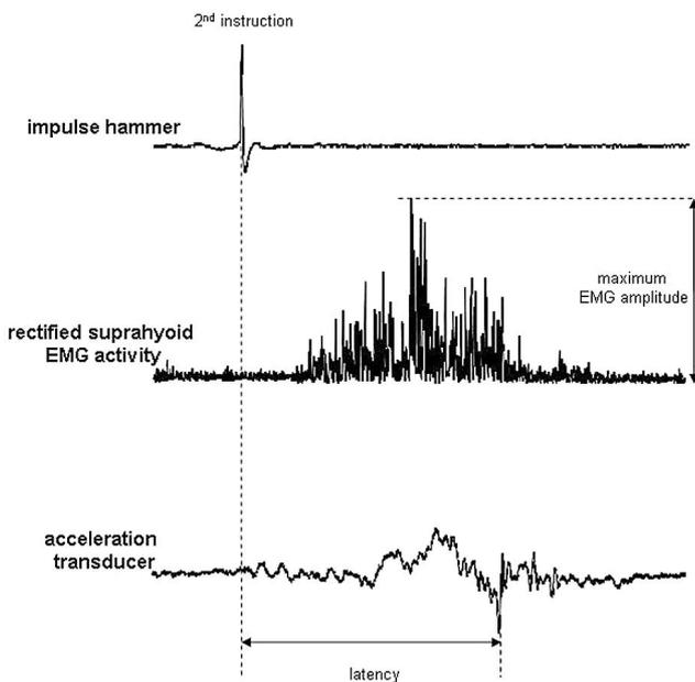
**Fig. 2.** A schematic illustration of the analysis of swallowing behavior in Experiment 1. Suprahyoid electromyographic (EMG) activity was full-wave rectified. See Experimental procedures for definitions of maximum EMG amplitude and latency to swallow.
