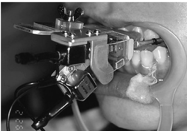
Figure 2. Measurement of tooth displacement with the two-dimensional tooth displacement transducer type K.
