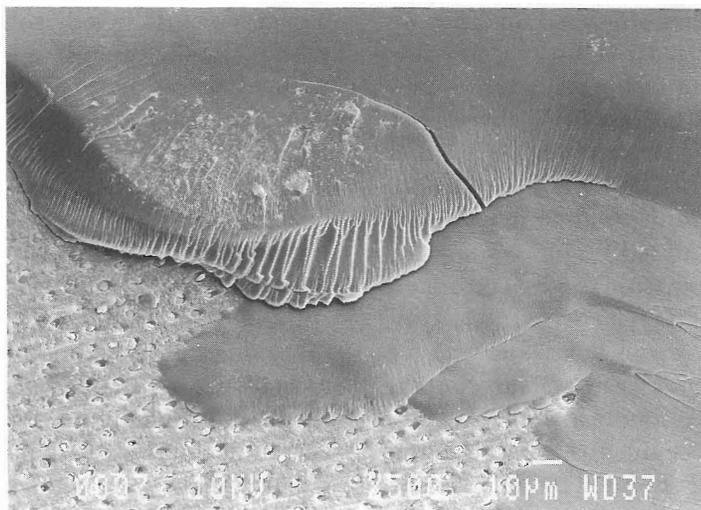
Fig. 6 SEM photograph of a six month specimen from Group LB. A combination of adhesive failure between resin and tooth, and adhesive/cohesive failure between the layers of bonding resin, Protect Liner, and resin composite can be detected.
