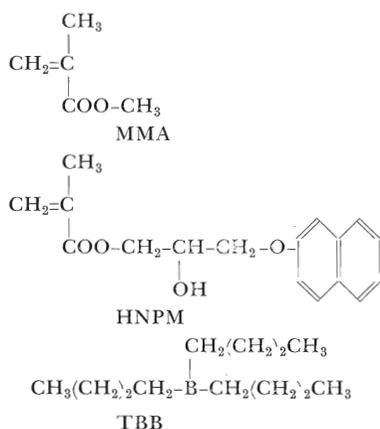
Fig. 1. Chemical formulas of MMA, HNPM, and TBB derivative.
